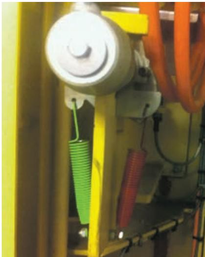
Both springs must always be replaced simultaneously.
