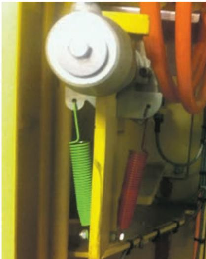
Both springs must always be replaced simultaneously.
